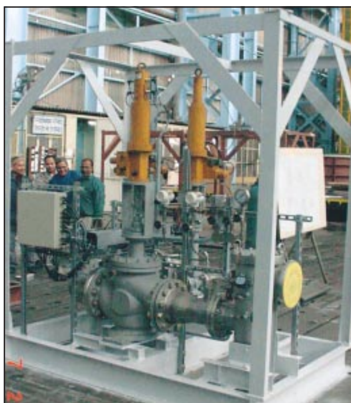
The fuel gas package assembly
