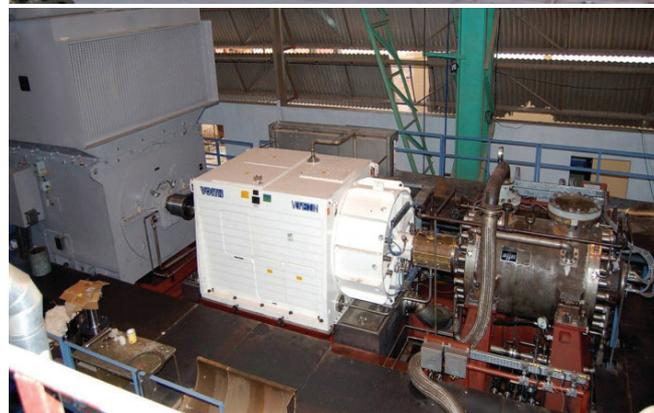
String test of Natural Gas Compressor driven by Job Motor for Marmul, Oman
