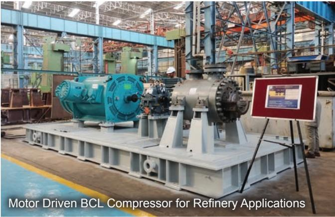
Motor Driven BCL Compressor for Refinery Applications
