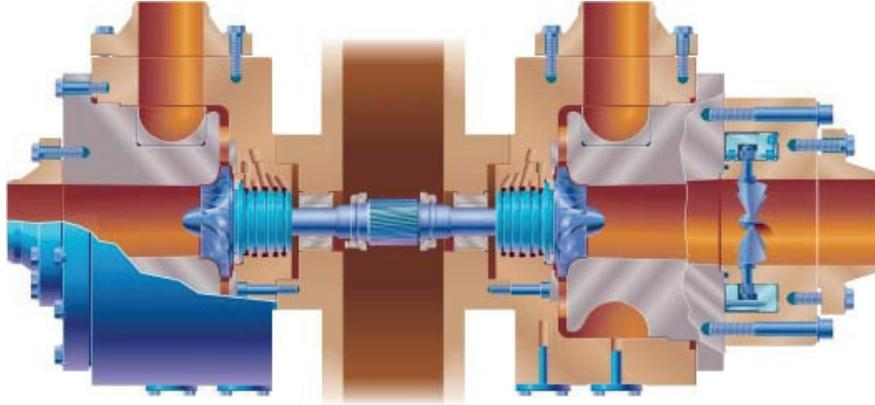
Integrally Geared Compressors are used in several petrochemical applications, either for low-flow/high pressure, or high-flow/low pressure conditions. This type of compressor has a bull gear and from one to four high speed pinions.
