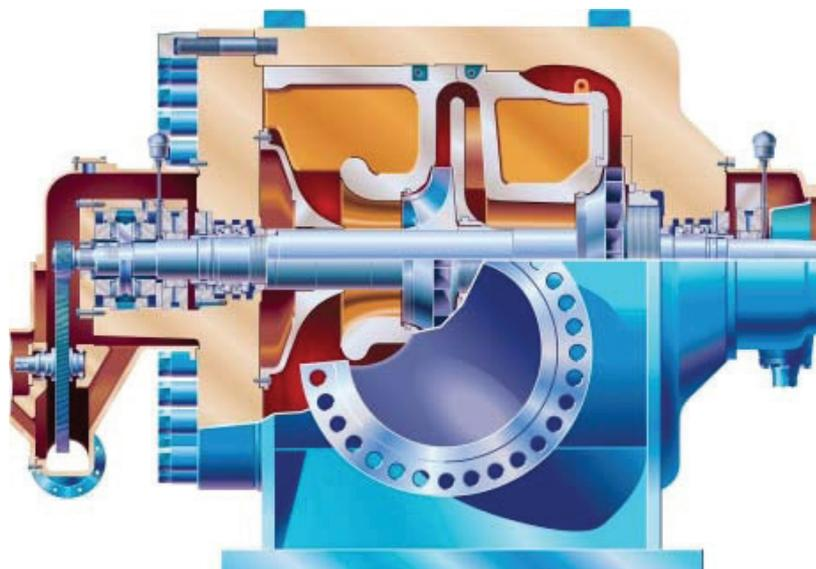
These compressors have been designed to meet the range of flow and compression ratios required by gas transportation stations.
