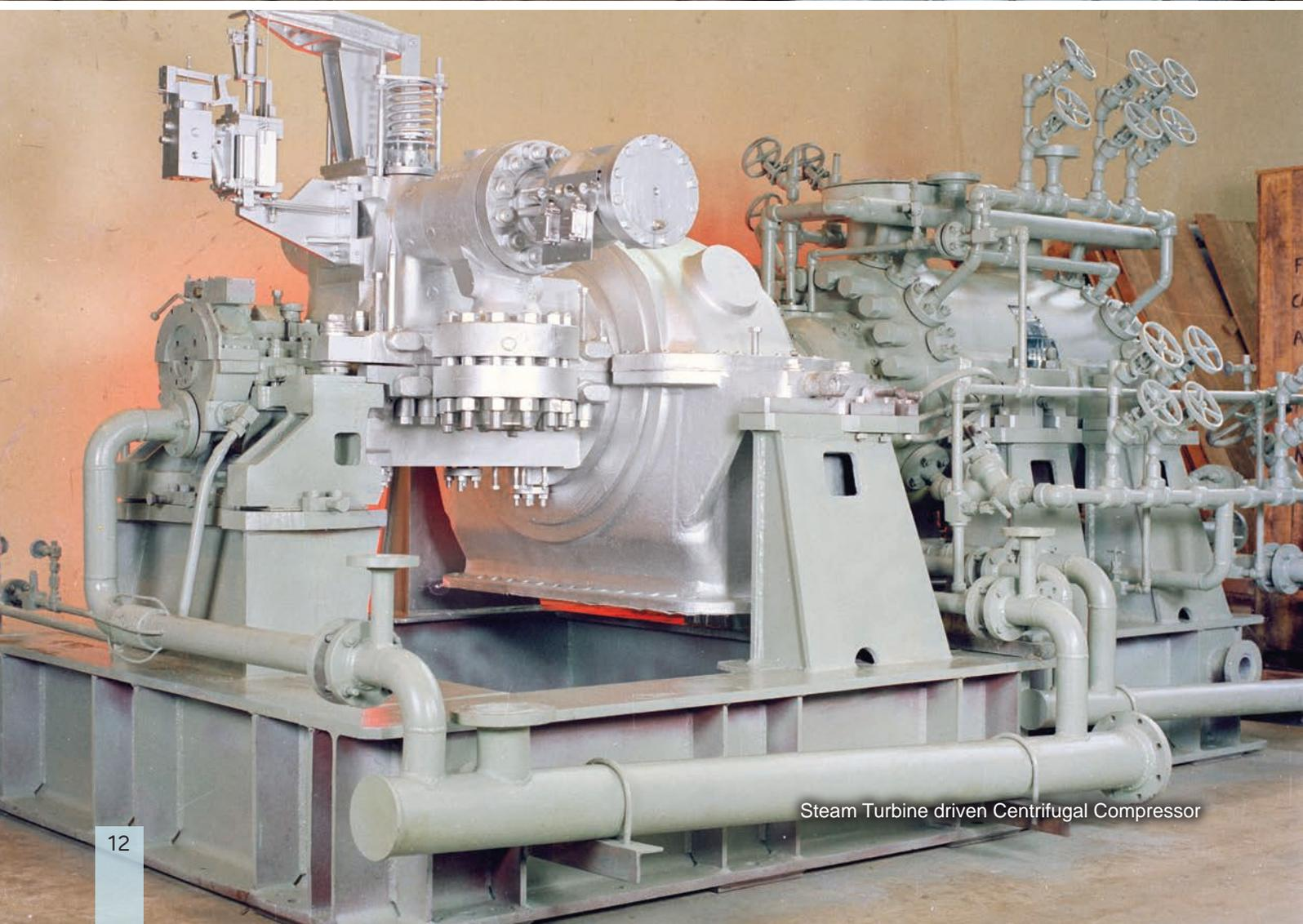
Steam Turbine driven Centrifugal Compressor
