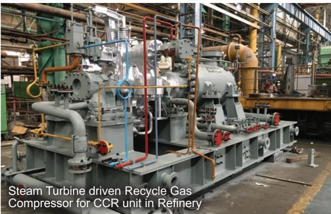
Steam Turbine driven Recycle Gas Compressor for CCR unit in Refinery
