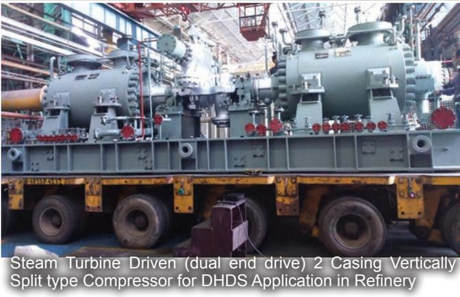
Steam Turbine Driven (dual end drive) 2 Casing Vertically Split type Compressor for DHDS Application in Refinery
