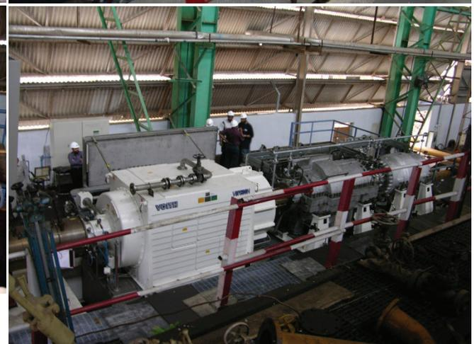
String Test of Gas Lift Compressor train driven by Motor for Lekhwair, Oman
