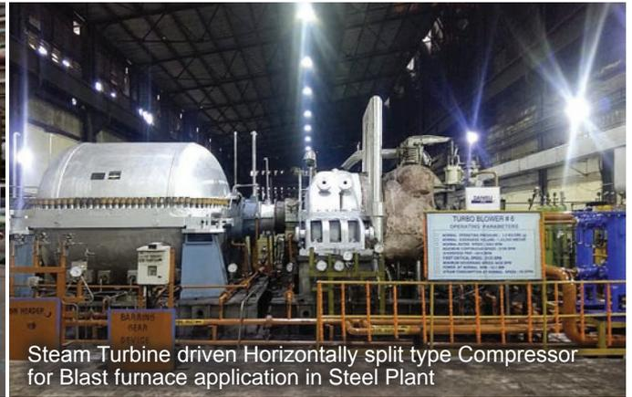
Steam Turbine driven Horizontally split type Compressor for Blast furnace application in Steel Plant
