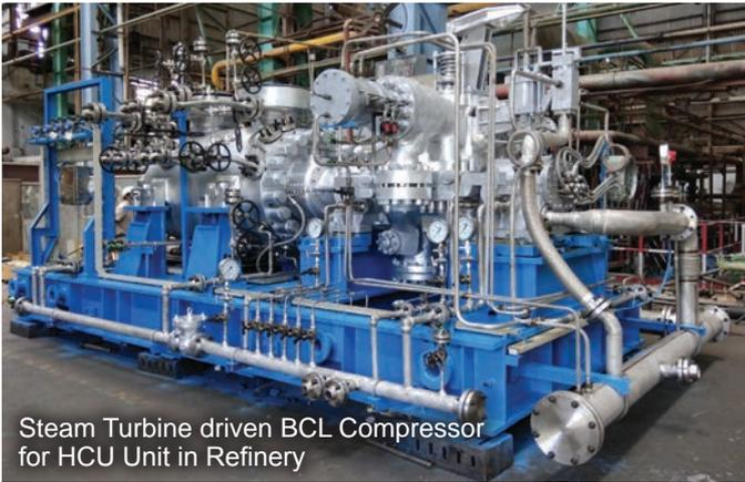
Steam Turbine driven BCL Compressor for HCU Unit in Refinery
