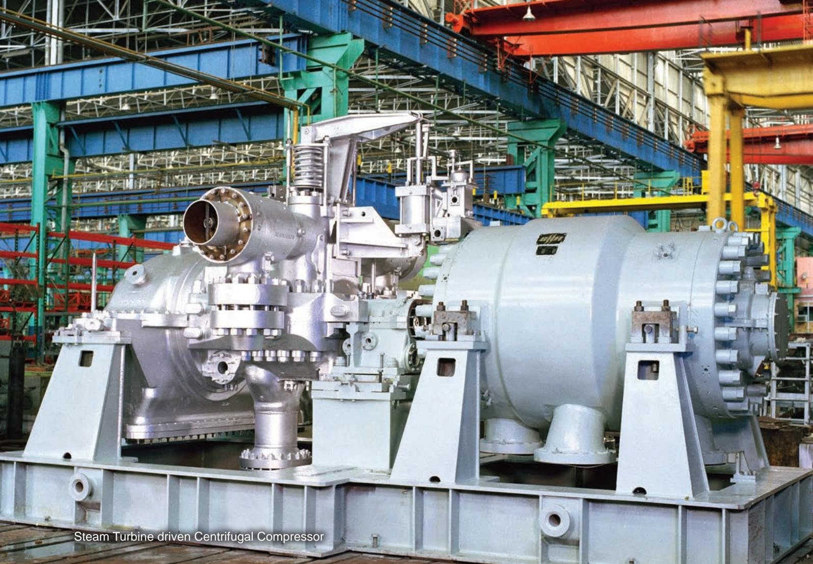
Steam Turbine driven Centrifugal Compressor
