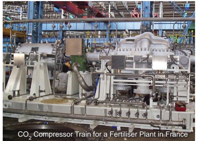
CO<sub>2</sub> Compressor Train for a Fertiliser Plant in France
