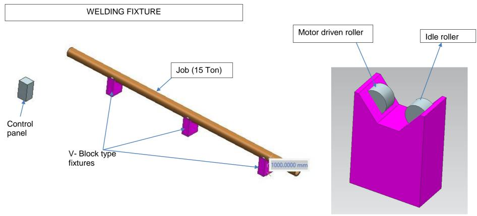
Note: The three motor driven rollers of three v-block type fixtures are VFD synchronized (Synchronous motion)
