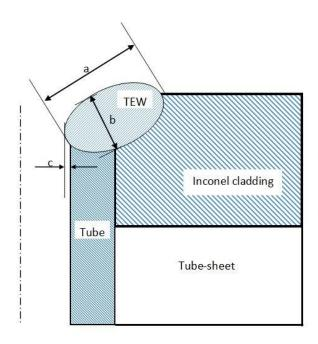
a = width of the weld (~=4.8mm)
