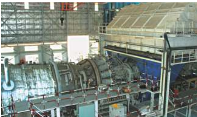
India's first indigenously built 9FA (250 MW ISO) Gas Turbine set manufactured by BHEL
