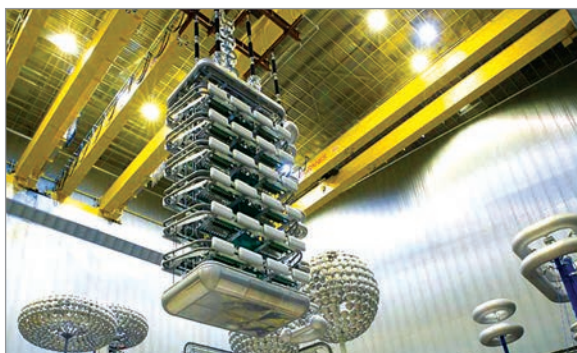
Thyristor Valve modules under Di-electric testing for \pm 800 kV, 6000 MW NE-Agra HVDC Project
