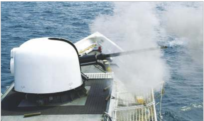
Super Rapid Gun Mount (SRGM) mounted atop naval ship
