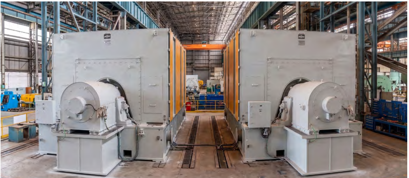
BHEL's highest-rated air-cooled Synchronous Generators - 4 nos 175 MW Generator manufactured for Jindal Mmamabula Energy Project, Botswana
