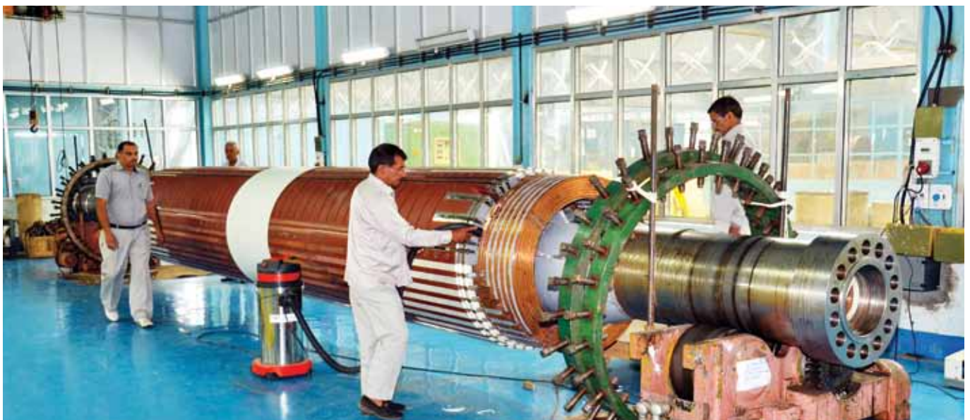
800 MW Turbo Generator rotor under assembly at HEEP, Haridwar
