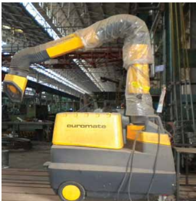
Introduction of mobile fume extractors in welding areas for sending out the welding fumes and metallic dusts at HPEP Hyderabad Unit
