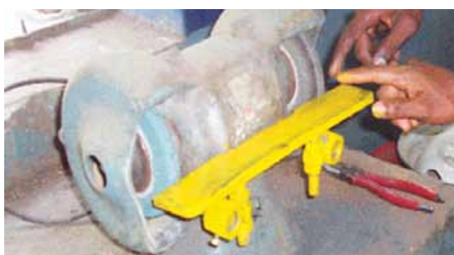
Adjustable tool rest fitted in pedestal grinder at BAP Ranipet unit
