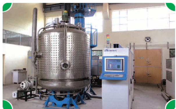
Plasma Nitriding System at Corporate R&D, Hyderabad
