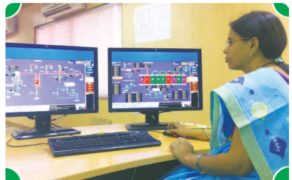
HRSG Training Simulator developed by Corporate R&D
