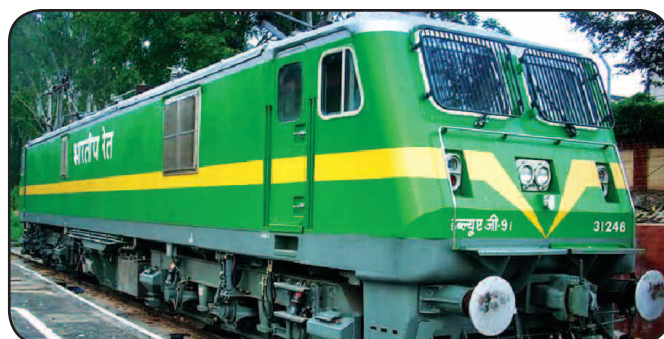
6000 hp electric locomotive of CLW equipped with BHEL's IGBT-based traction & auxiliary converters
