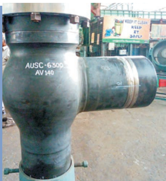
HP Bypass Valve with Nickel-based Alloy for Advanced Ultra Supercritical (AUSC) Power Plant Application Developed at BHEL Tiruchirappalli
