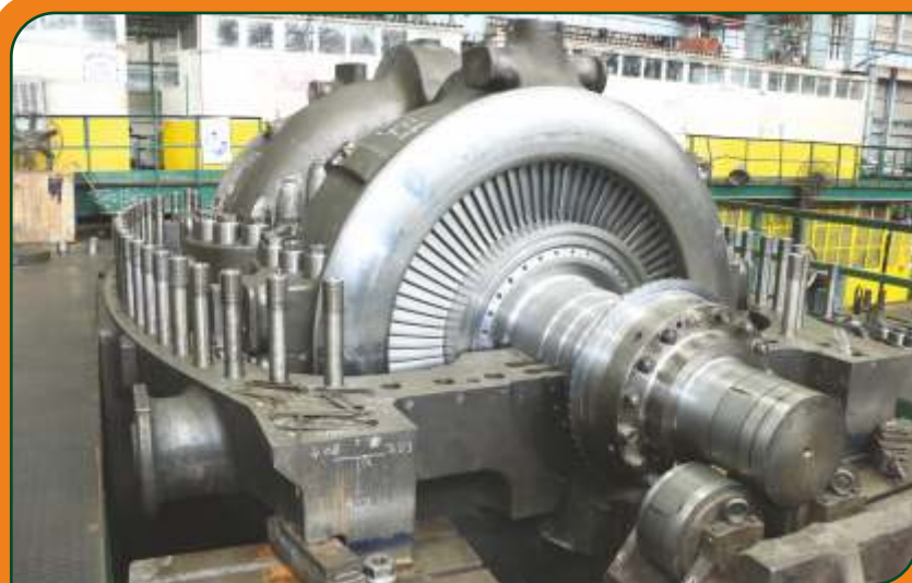
800 MW IP Turbine under assembly at BHEL works for NTPC
