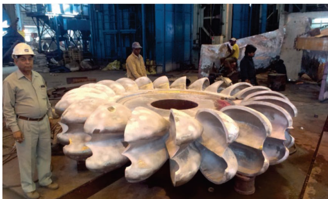
Pelton Runner casting
