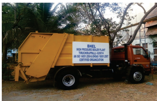
Figure 56: 4 MT Garbage Compactor with 80 Nos. 1100 Litre MS Compactor bins at Trichy
