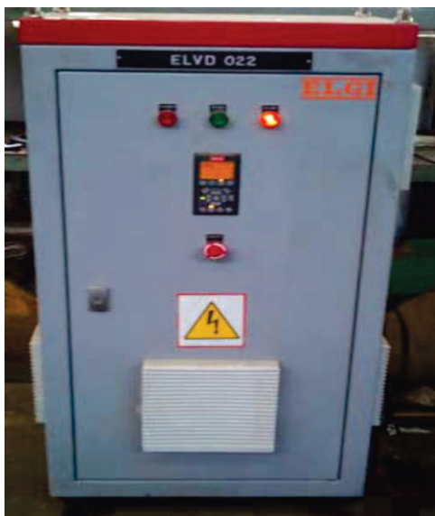
Figure 33: Replacement of welding rectifiers by welding inverters at BAP Ranipet
