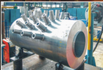
BHEL has successfully fabricated mock up Thick-Walled Superheater Header for AUSC Boilers with Advance High Temperature Materials
