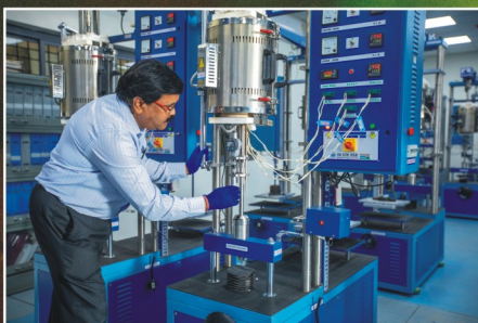
Creep Testing Machines for testing of Advanced Materials for AUSC Power Plant Applications.
