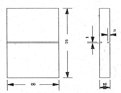
FIGURE: 1-LIQUID PENETRANT COMPARATOR BLOCK
