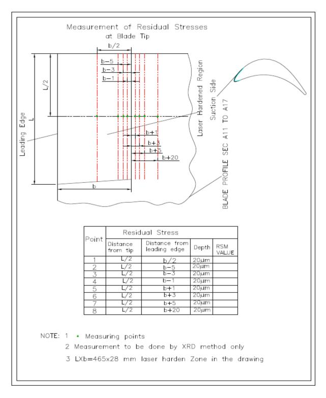
Figure D: Laser harden region and position / measuring points for residual stress measurement at Suction side of blade profile.
