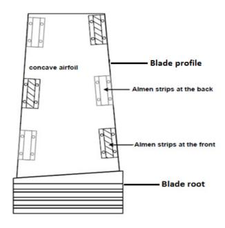
Figure A: Position of Almen strip at the blade profile
