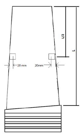
Figure C: Positions of residual stress measurements at suction and pressure side of blade profile.
