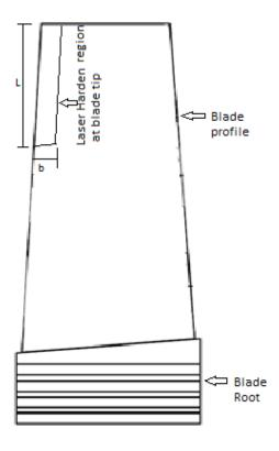
Figure B: Position of Laser harden region in the blade drawing
