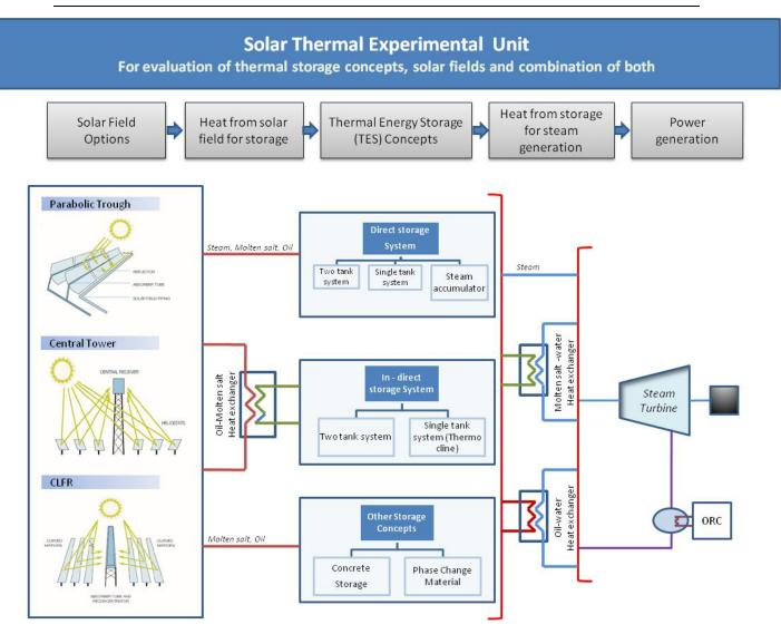
Figure 1. Schematic of Solar Thermal/CSP Experimental Plant
