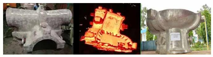
World's heaviest and largest casting in Alloy 625 grade (IP Inner Casing LH – 21 MT & UH – 9MT) for AUSC mission project manufactured at CFFP Haridwar
