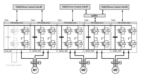
The damping resistor will absorb the high frequency components in the inverter output generated as a result of IGBT switching. A ferrite core assembly is provided at the output of the auxiliary inverter which will trap the high frequencies which are dissipated by the damping resistor.
