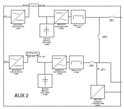
Load changeover in case of isolation of any one of the converter is done automatically by the auxiliary converter electronics with the aid of contactors.
