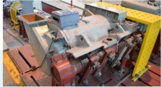
3 – Phase AC EMU Motor – 285 kW
