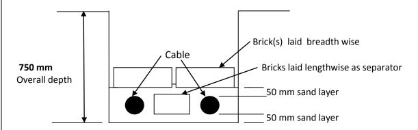
The cables should be laid in horizontal plane. The **trench should be excavated** to a depth and breadth, such that the cables will be laid at a **minimum depth of 750 mm in horizontal plane** as shown above. Spread 50 mm deep layer of sand below the cables. Lay the cables in horizontal plane & place **good quality bricks** in between **them <u>length wise</u> continuously all along the cable / trench.** Further sand filling to be done for 50 mm over the cables.
