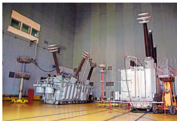
Power transformers under testing at BHEL's Ultra High Voltage Laboratory in Bhopal
