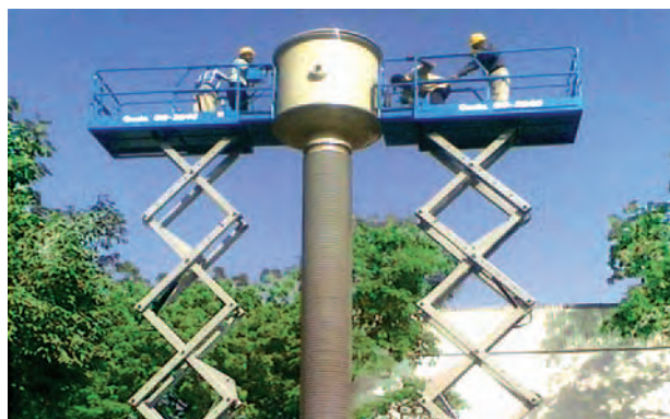
Prototype of 765 kV gas-insulated current transformer developed in-house at Corp. R&D
