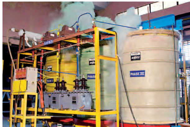
1 MVA, 3-phase, 33/6.6 kV, HTSC Transformer
