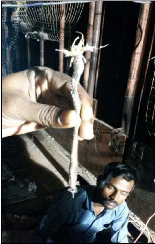
Figure B3.2: K - Type Thermocouple
