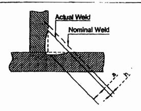
A fittet weld with an apparent throat thickness smaller than that prescribed should not be regarded as being imperfect if the actual throat thickness with a compensating greater depth of penetration complies with the nominal value.
